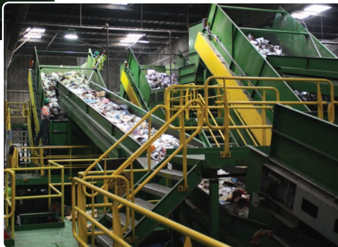
MSW is delivered to the tipping floor at the GreenWaste MRF (above). Mixed paper and other lightweight organic materials are separated from recyclable containers at the polishing screen on the MSW line (right).
